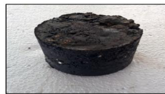
Marshall Stability sample with Samanea saman fruit
